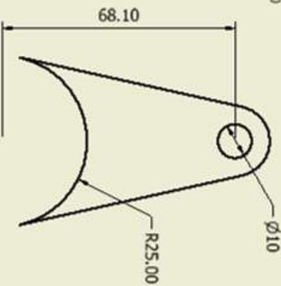
SUSPENSION AXLE LEVER (SIDE VIEW) (1 : 1)
