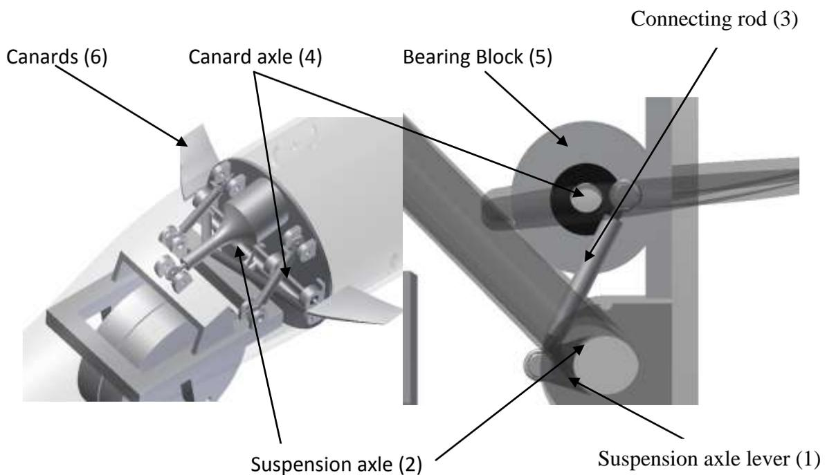
At high speeds, the system may experience excessive vibrations of the canards due to fast moving terrain. This could cause a fluttering effect producing unwanted lift. To solve this problem, our team proposes that we use a damper in series or parallel with the connecting rod to control or minimise canard vibrations. The damper should also reduce cyclic induced force and allow the canards to only respond to generalised terrain undulations.
